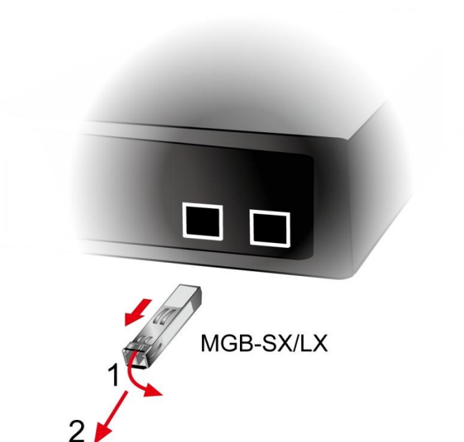
Figure 2-17: How to Pull Out the SFP/SFP+ Transceiver
